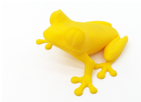
Pict. 28 - the 50-microns treefrog is commonly used as a 3D printing benchmark.
